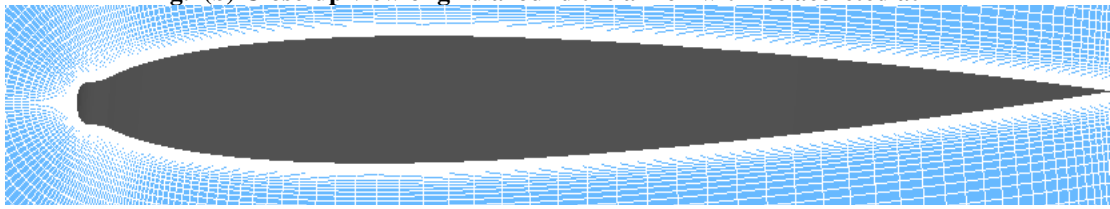
Fig.4(b) Close-up view of grid around the airfoil with ice accreted at LE
