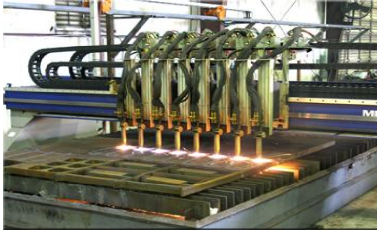
Fig.no 1.2 Flame cutting operation
