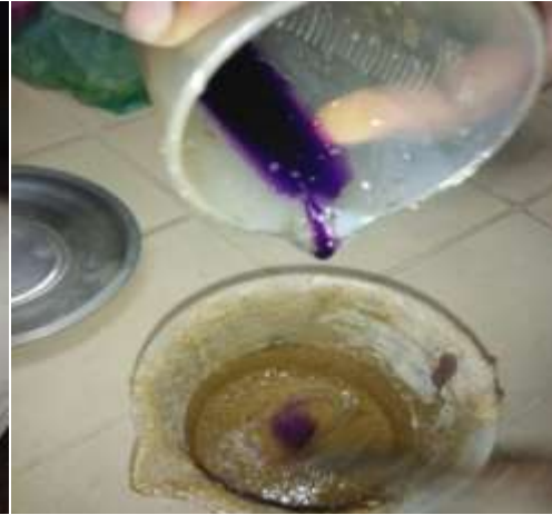
Figure 9 Mixing the Accelerator
