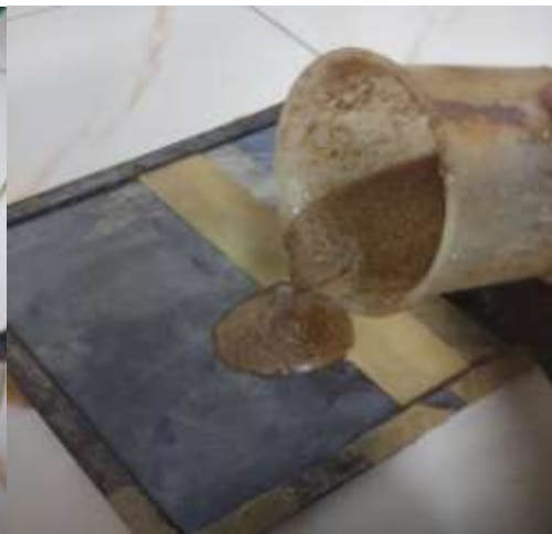
Figure 11 Pouring the mixture into the Mould
