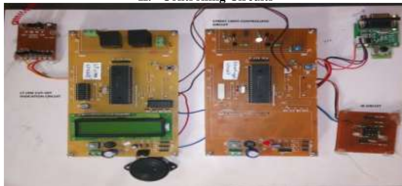
Fig2. controlling circuits for street lights and Lt line cut-off indication
