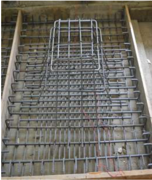
Fig (3): Details of Specimens Casting Forms Fig (4): pouring concrete in slabs
