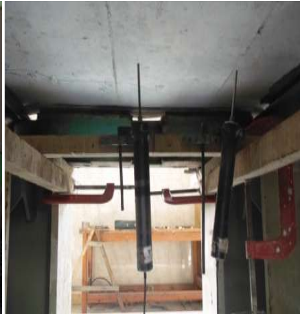
Fig (7): Locations of vertical LVDT'S
