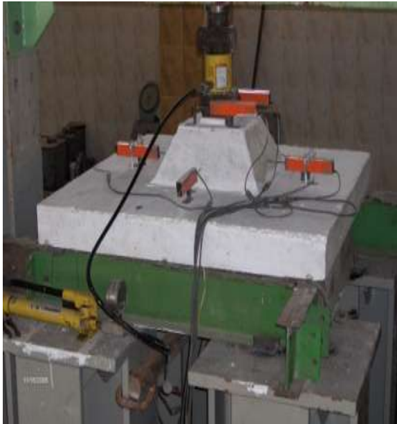
Fig (6): Locations of vertical LVDT'S
