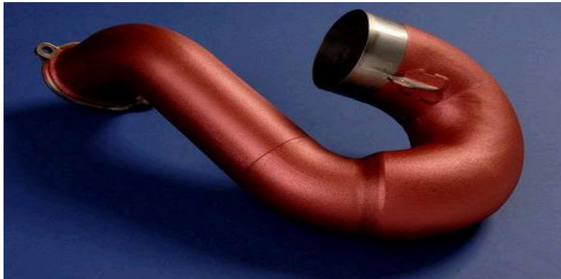
Figure 1. Thermal barrier coating applied onto automotive exhaust system
