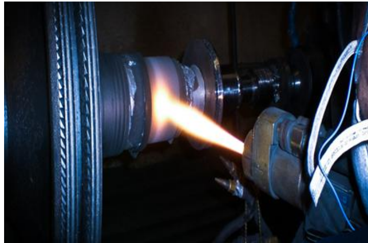
Figure 5. Plasma Spray Process
