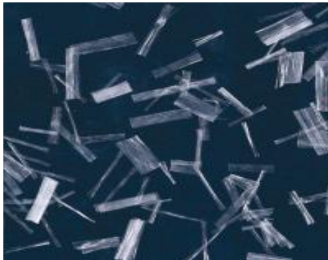
Fig 1.1 Fibermesh 300-E3 Micro Synthetic Fiber
