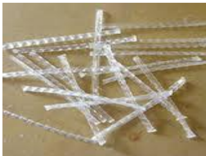
Fig 1.2 Fiber Tuff Macro Structural Synthetic Fiber
