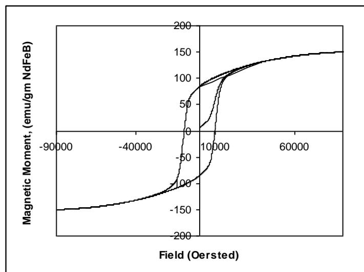
Fig. 1 Complete M-H plot of a NdFeB sample
