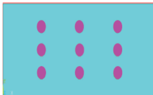
Figure 3.2 Fem model of the composite with fiber and matrix
