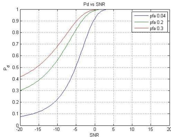
Fig. (6)  $P_d$  vs. SNR for different  $P_{fa}$
