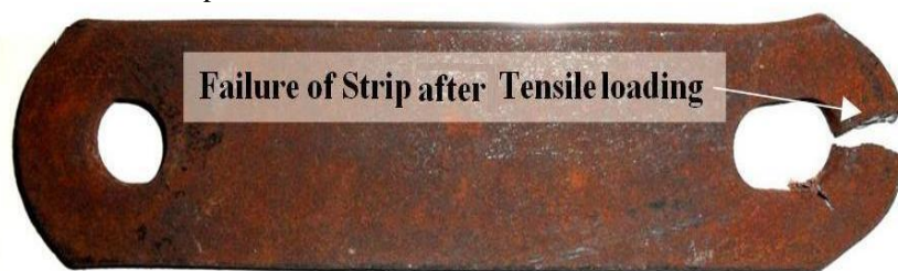
Fig.6 Failure of Strip
