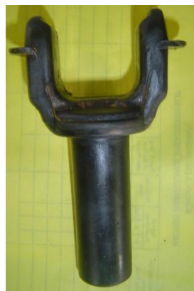
Fig. 6 a (Near net shape Forged Part)
