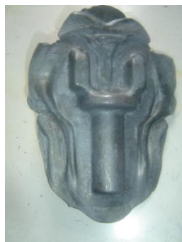
Fig (2b) Drop forged part
