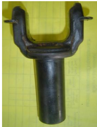
Fig (5e) Stage -4 (Finished yoke)
