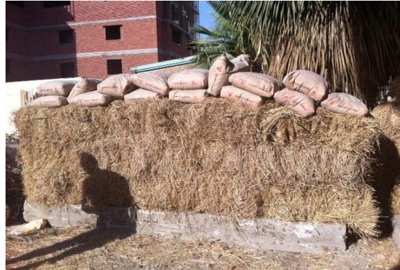
Figure 2: Pre-compression Test of full scale wall A
