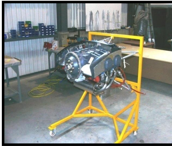
Fig. 8: Lycoming O-320-B Engine on Test Bed
