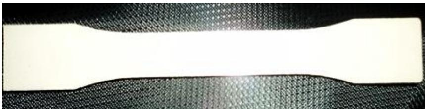
Fig: Tensile specimen As per ASTM D638
