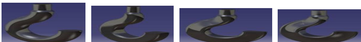
Fig. 3.1 Circular, Square, Curved and Modified Curved cross section Hook
