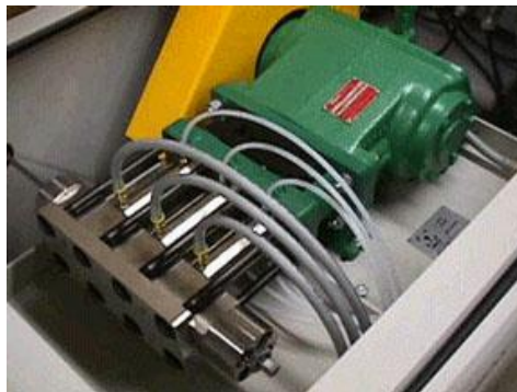
FIG: 2 Typical 20/30 horsepower crankshafts driven triplex pump.
