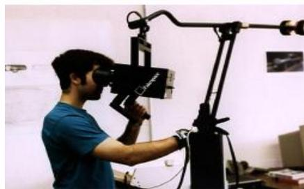
**Figure. 4.** BOOM (Binocular Omni-Orientation Monitor)
