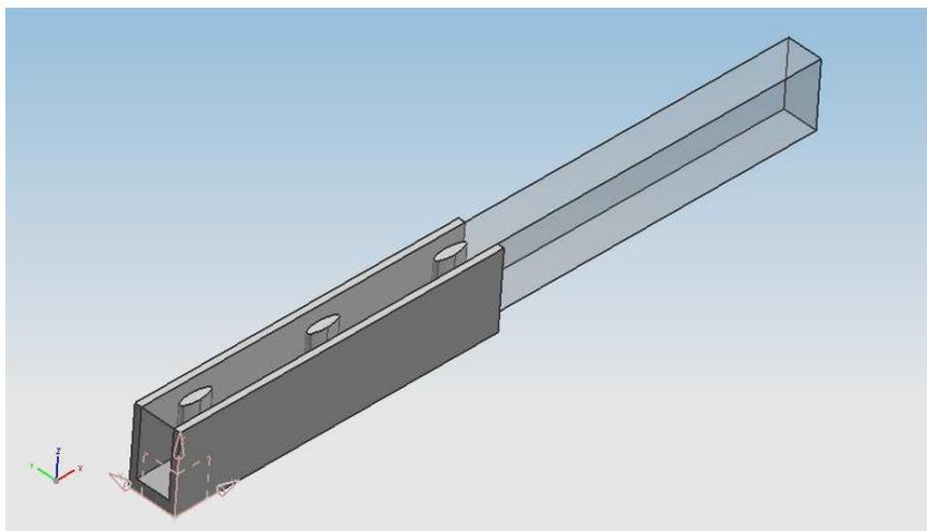
Fig.3 Model of 2.0 Elliptical pin-fin Heat sink
