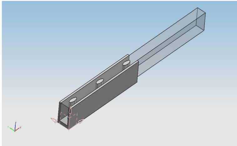
Fig.2 Model of 1.5 Elliptical pin-fin Heat sink
