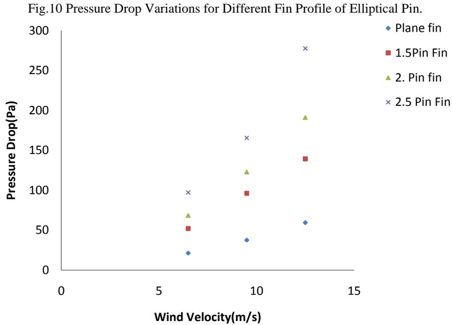
The above Fig.10 the Pressure drop variations for different fin profile of elliptical pin with compare the plate fin result(7) of PFHS and simulation result of various fin profile of elliptical pin gives a constant deviation in elliptical fin pin heat sink but in similar manner of experimental results. This fig. shows the increase in the pressure drop with increase the wind velocity (6.5, 9.5 & 12.5m/s)
