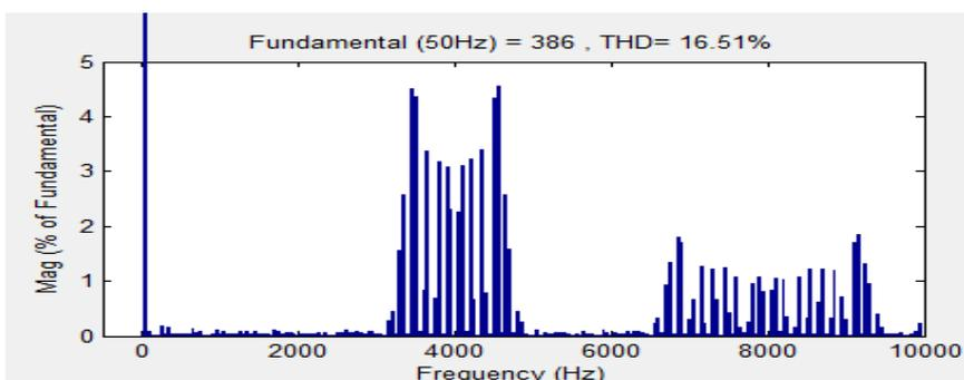
Fig .10.THD values of phase disposition PWM technique
