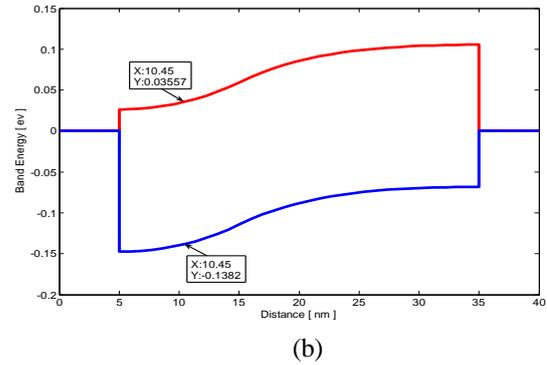
Fig. 4. (a) I-V characteristic and (b) band diagram of InSb PN Junction at 300°K
