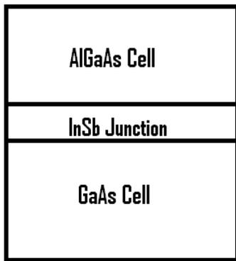
Fig. 3. New structure for tandem solar cell
