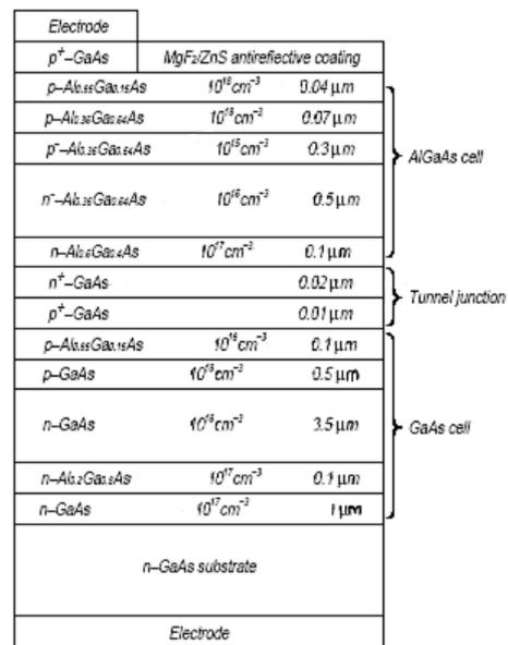
Fig. 1. A double junction AlGaAs/GaAs tandem solar cell with 28% efficiency
