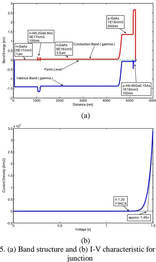
Fig. 5. (a) Band structure and (b) I-V characteristic for GaAs junction
