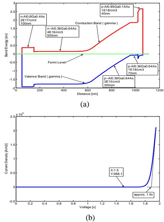
Fig. 6. (a) Band structure and (b) I-V characteristic for AlGaAs junction
