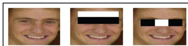
Figure 2. Examples of Haar features. Areas of white and black regions are multiplied by their respective weights and then summed in order to get the Haar feature value.
