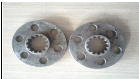
Fig.1 Specimen (Plain carrier) of EN-8 material
