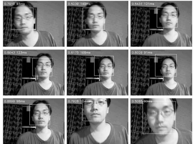
Fig.7. Face detection demonstration when we used a camera. Numerals on the left-upper are respectively the maximum value of a cost function and computational cost value for each frame.
