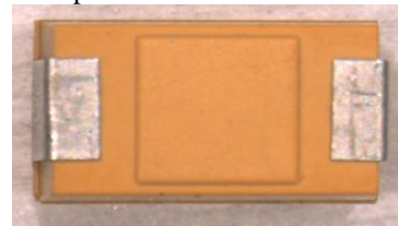
Figure 1. Bottom side of a surface mount tantalum capacitor used in this research.
