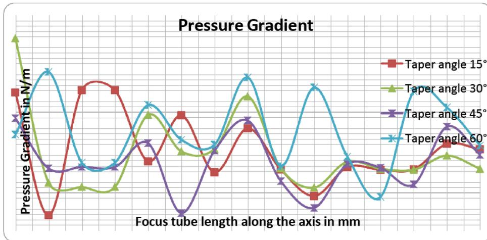
Figure 6 (b) Pressure gradient in the focus tube
