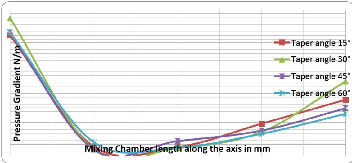
Figure 6 (a) Pressure gradient in the mixing chamber
