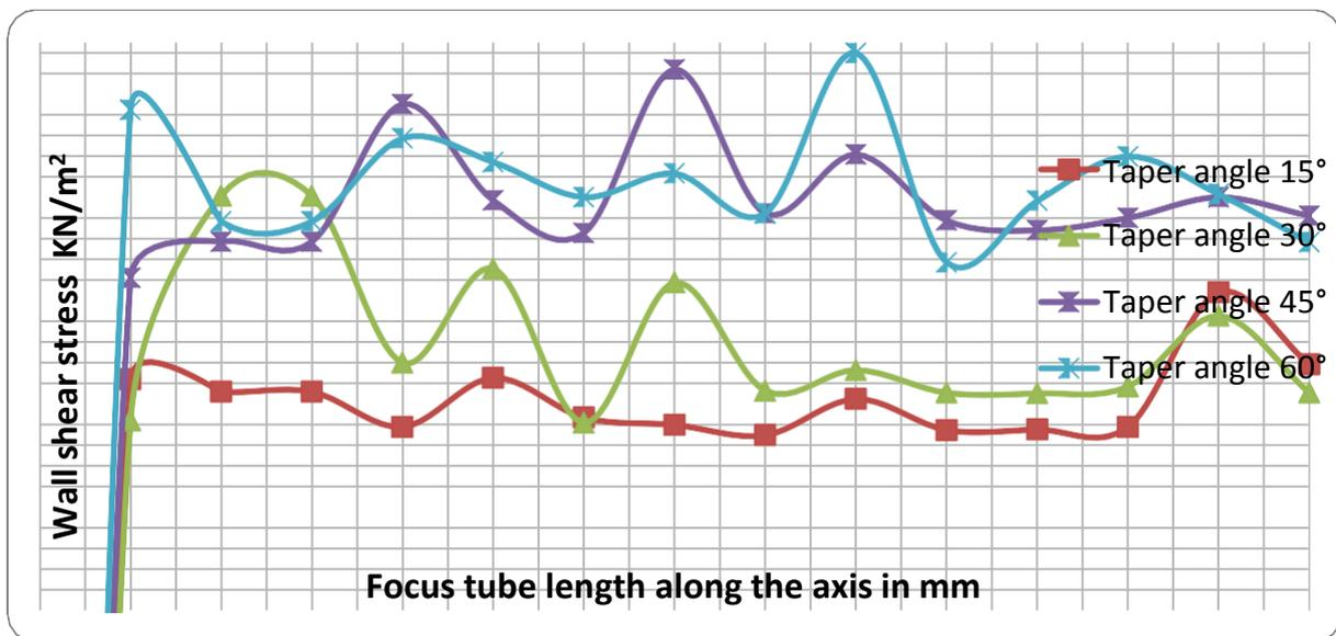
Figure 5 (b) Wall shear stress along focus tube
