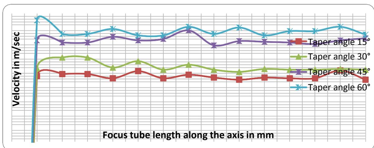
Figure 4 (b) Velocity variation along the Focus tube
