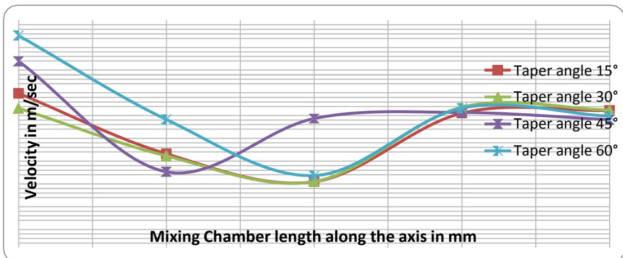
Figure 4 (a) Velocity variation along the Mixing Chamber
