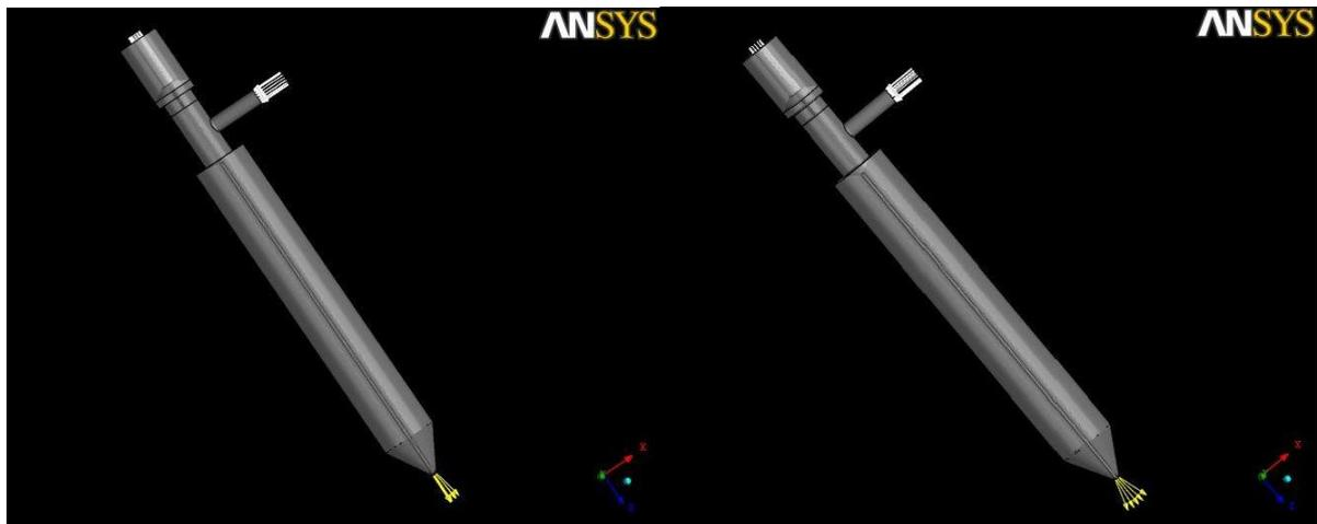
**Figure 3** Computational Domain of nozzle with taper angle of 45° and 60°
