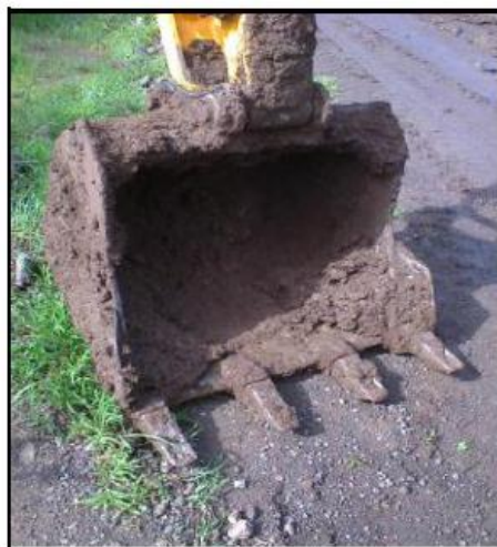
Figure 1: Bucket with adhered soil
