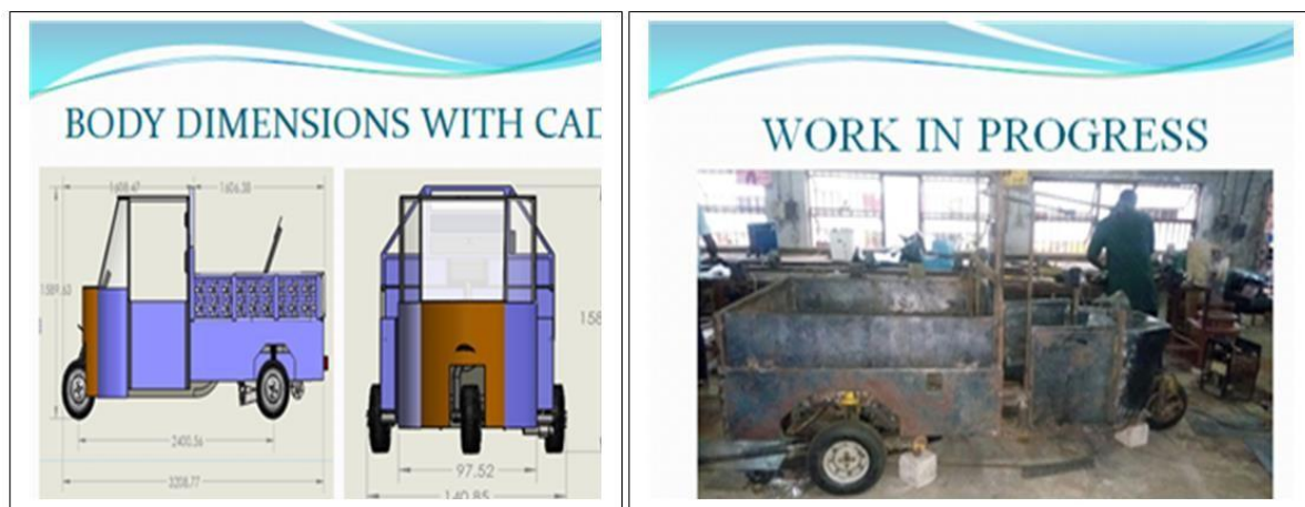
Figure 12: Body dimensions of the tricycle and work in progress
