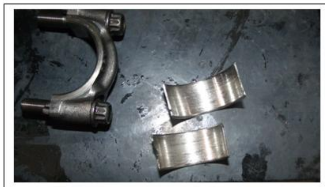
Figure 3 - Connecting rod bearing of the 3rd cylinder.
