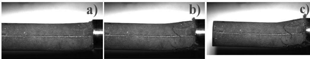
Figure11b: Development of the specimen damage during impact loading of the specimen. Material A. Striking velocity 27 m/s.
