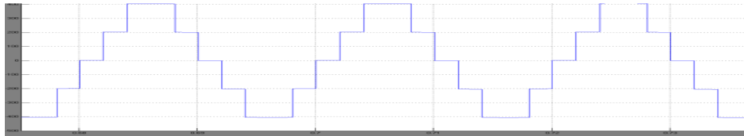
Figure12. Five level output of Hybrid H-bridge
