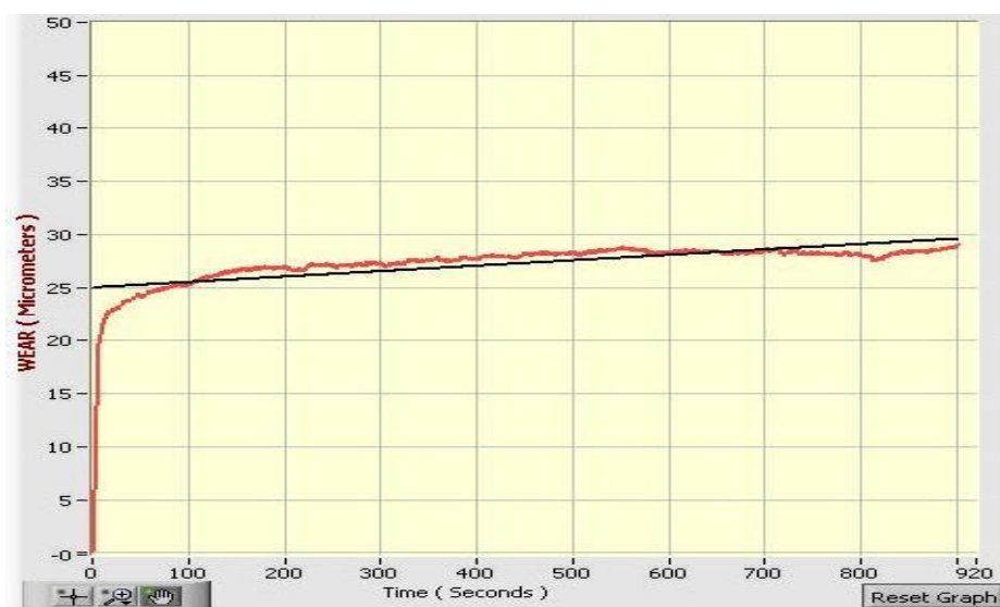
Fig.14. Wear (Micrometers) V/s Time (Seconds) at load 20N for 20wt% \text{Al}_2\text{O}_3
