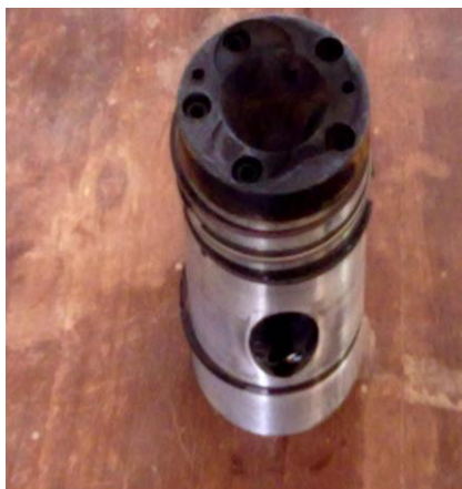
Fig. 1: Photographic view of Aluminum piston Crown with an air-gap insulation
