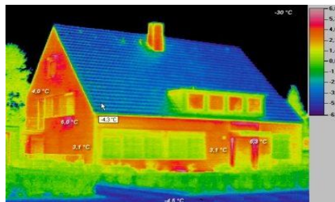
Fig 4: captured image by thermal imaging system
