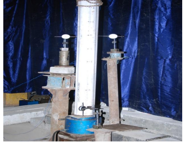
Fig.3.2 Dial Test Indicators laterally & axially
