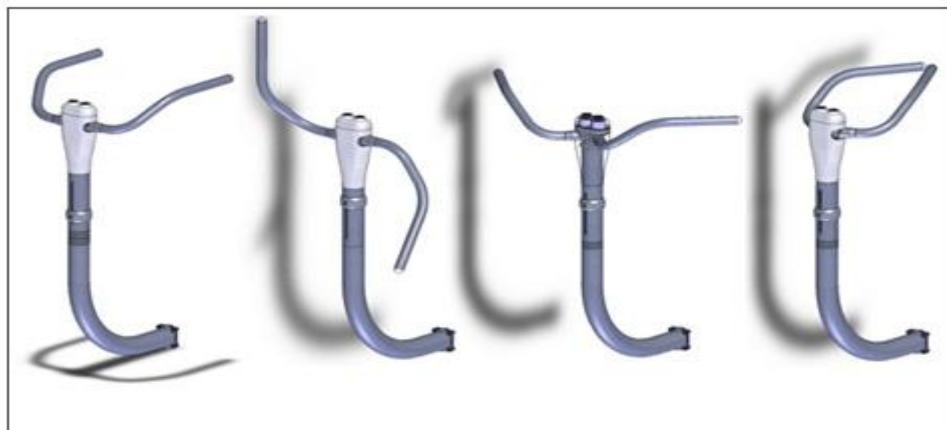
Fig. 1 Illustration of the mechanical add-on device and its movement options
