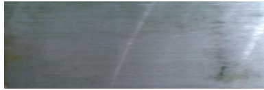
Fig V: Transverse cracks on observed after etching with HCL
