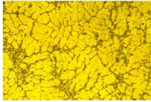
Fig12: 6Hz vibration without grain refiners
