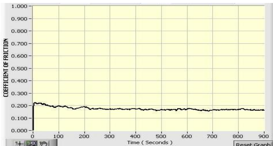
Fig.12. Coefficient of Friction V/s Time (Seconds) at loads 10N for 20wt% \text{Al}_2\text{O}_3
