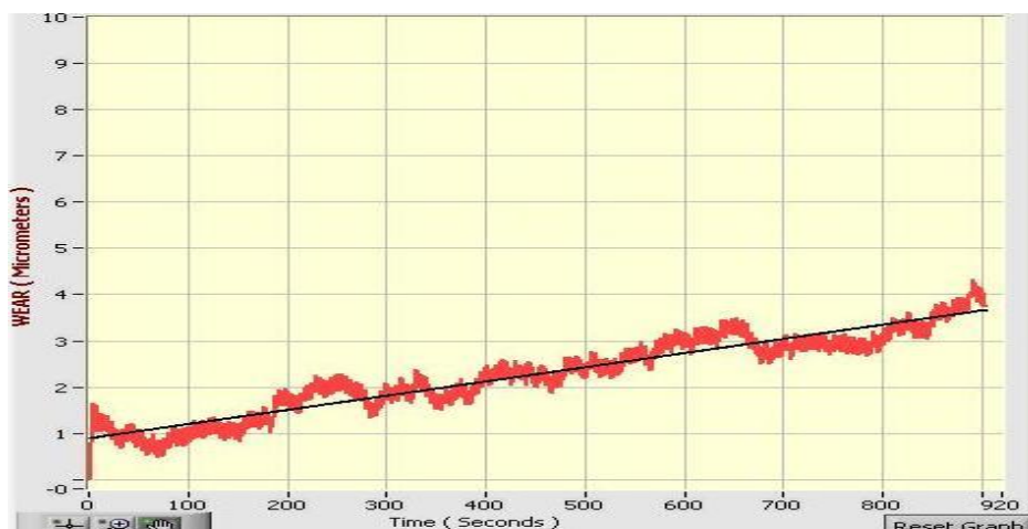
Fig.11. Wear (Micrometers) V/s Time (Seconds) at load 10N for 20wt% \text{Al}_2\text{O}_3
