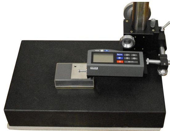
Fig. 2 The surface roughness measurement on a specimen using surface tester TR 200
