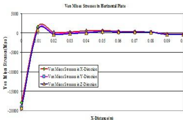
Figure-6: Von mises Stresses in horizontal Plate
