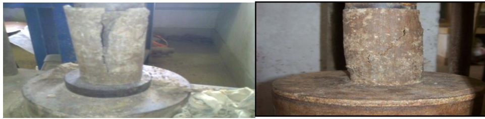
Figure 1: UCS Test - specimens crushed to total failure
