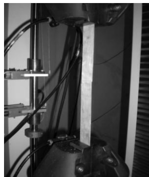
Figure 13 Specimen during tensile testing
