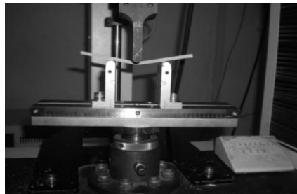
FIGURE 16 SPECIMEN DURING FLEXURAL TESTING
